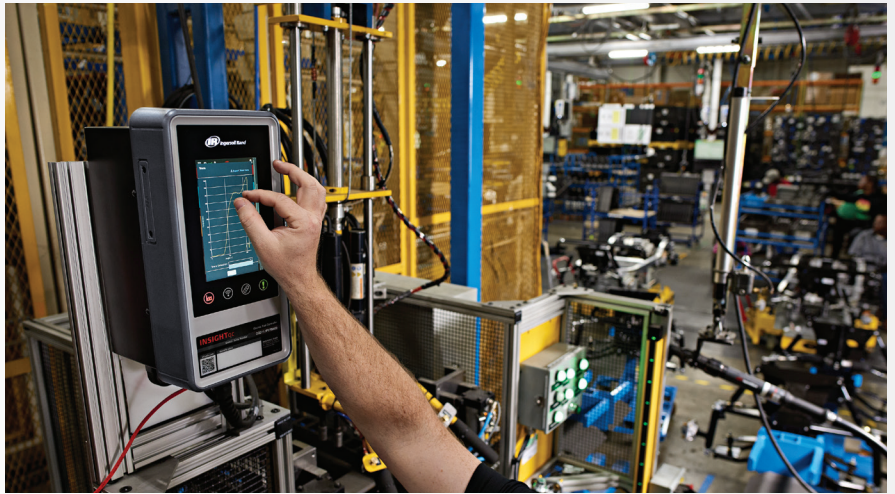
The Ingersoll Rand INSIGHTqc™ controller comes with plug-and-play hardware and software that works with your industrial protocol.
